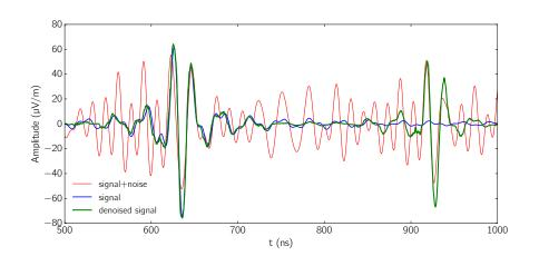
Signal-like RFI is identified as signal
