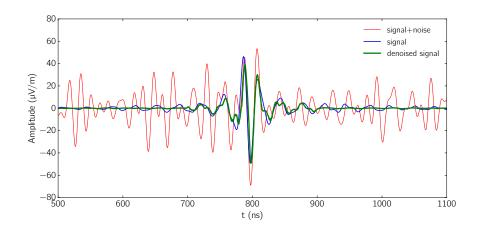
True signal and noise are identified correctly, noise is removed
