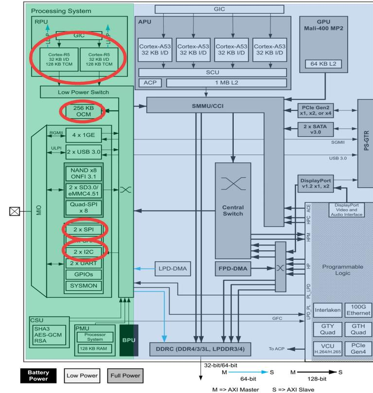
Figure 2-1: Zynq UltraScale+ MPSoC Device Hardware Architecture
