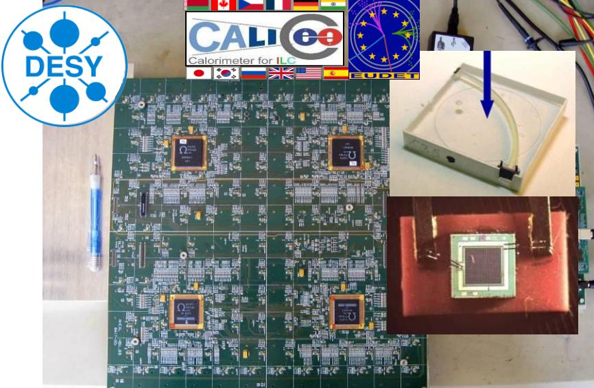
$(0.36m)^2 \text{ Tiles} + \text{SiPM} + \text{SPIROC (144ch)}$
