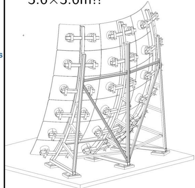
Hidden photons convert to light at a spare mirror system of the AUGER fluorescence telescopes, which is focused onto a photomultiplier.
