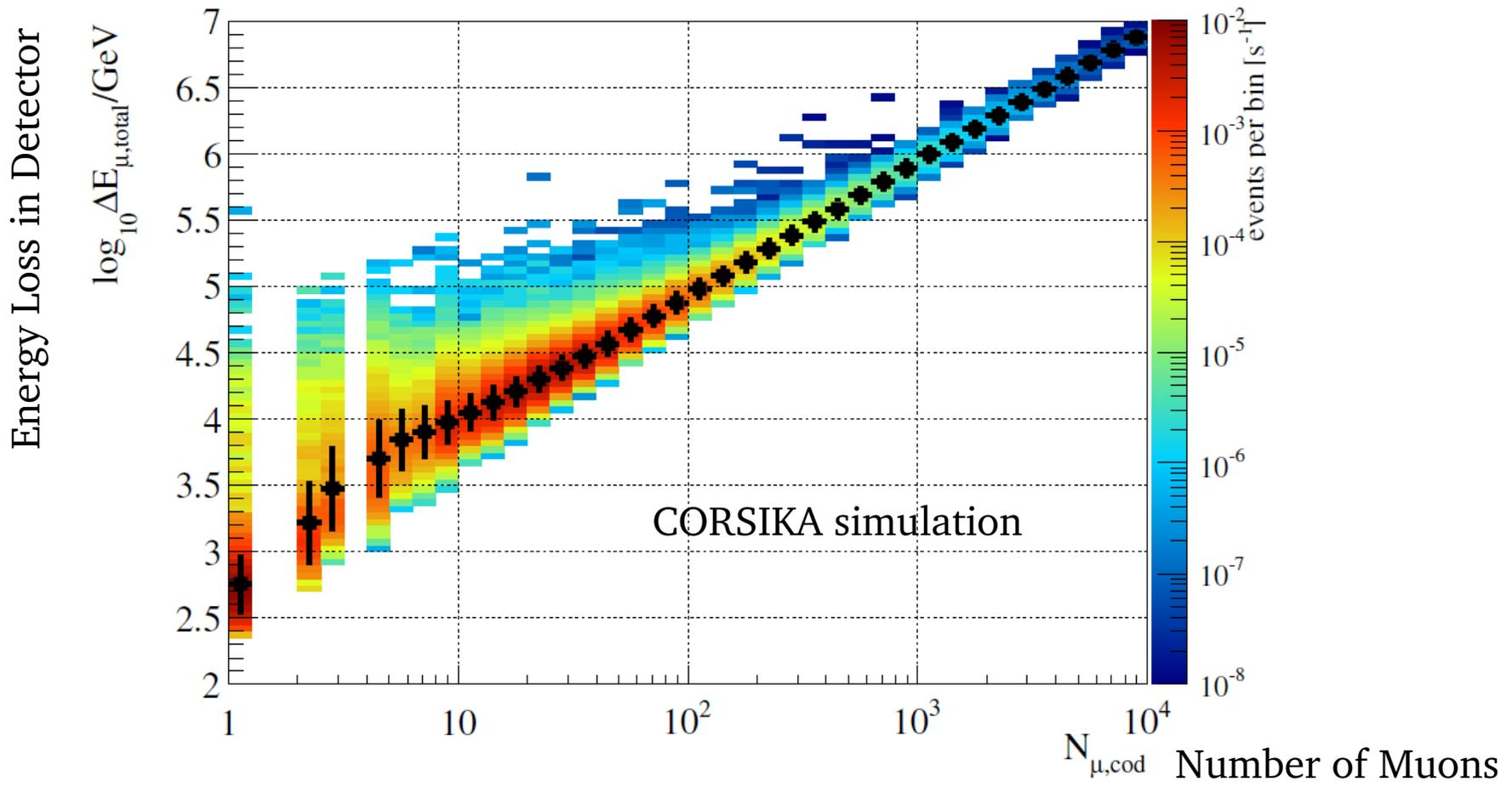
**Experimental Aspect:** After selection cuts, measurable energy deposition in detector is very closely related to number of muons.
