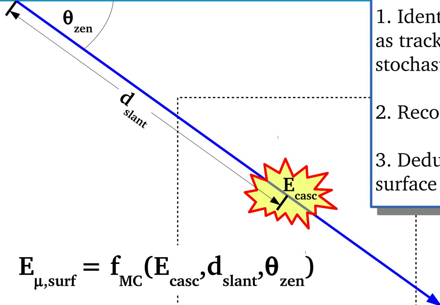
The diagram shows a blue line representing a muon track starting from the top left and extending towards the bottom right. The angle between the track and a vertical dashed line is labeled  $\theta_{zen}$ . The distance along the track is labeled  $d_{slant}$ . A yellow starburst with a red outline is positioned on the track, containing the label  $E_{casc}$  and a small black arrow pointing along the track. Dotted lines connect the starburst to the equation below and the list above.
