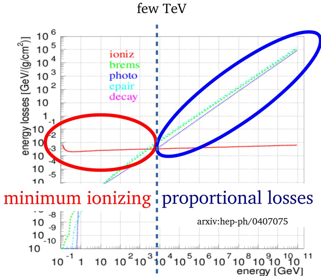
Simulated loss rates along muon tracks in IceCube detector for  $E^{-2.7}$  CR Spectrum
