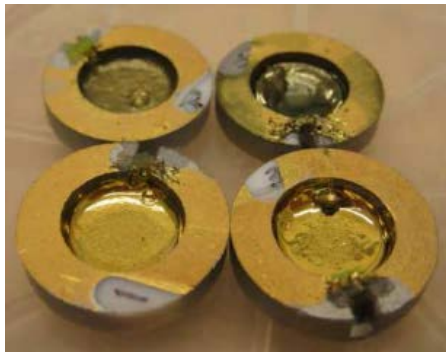
Detector 7 \text{ mm} \phi \times 5 \text{ mm} deep
